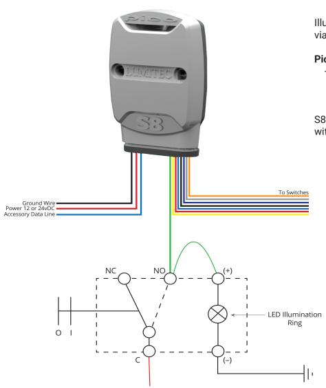
Illumination of switches is synchronized with digital control via App or MFD.
